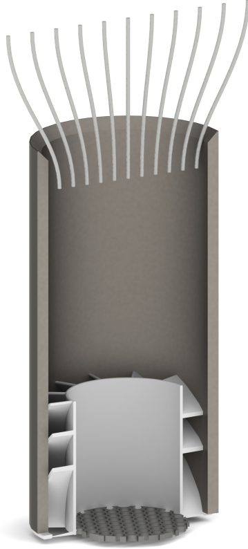
Figure 1.1: Schematic cross section of a low-swirl burner. The diverging flow field is illustrated by the streamlines at the burner exit.
