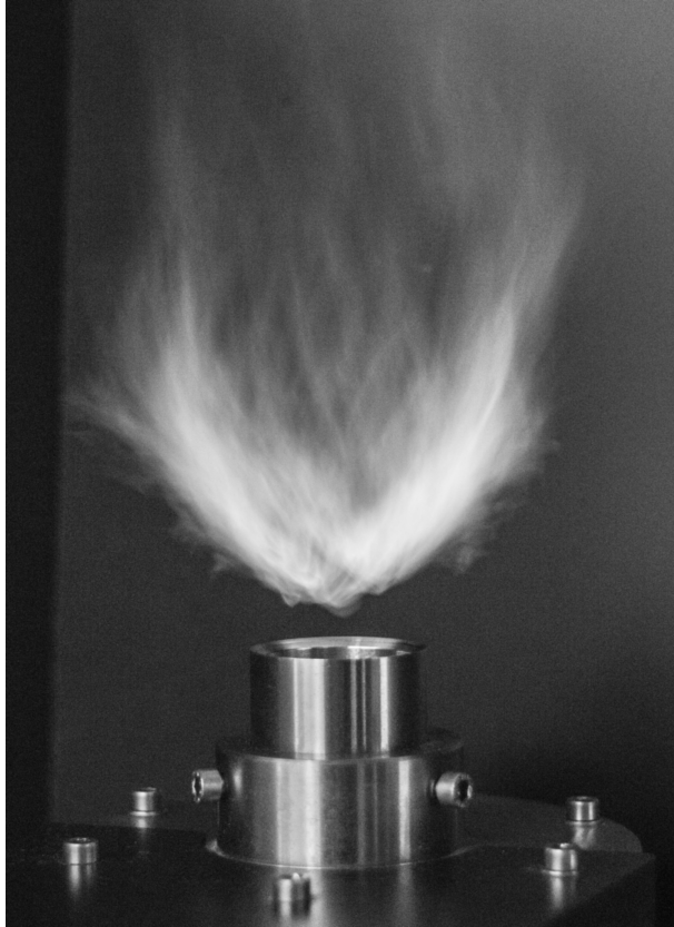
Figure 1.2: Photograph of a typical low-swirl flame. The inner tube diameter is 44 mm and the mean axial velocity is 8.4 m/s. As fuel Dutch natural gas is used at a thermal power of 33 kW. The photograph is taken using a shutter time of 1/100 s.
